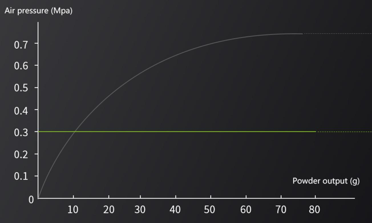
Ordinary airpolishing machines change the powder output by adjusting the air pressure, which causes uncomfortable such as tooth soreness during cleaning.
